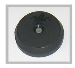
The T-Series of RFID Tags from Escort Memory Systems offers exceptional memory capacity in a very economical package. These 2 Kilobyte tags are passive: no batteries are required. Power to the tag is supplied inductively via the RF field when in the range of a compatible RFID controller.
